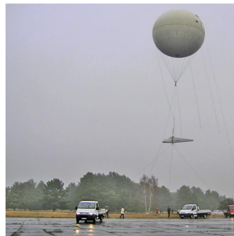
Successful test with a 1:8 scale model of the CargoLifter AirHook (2008)
