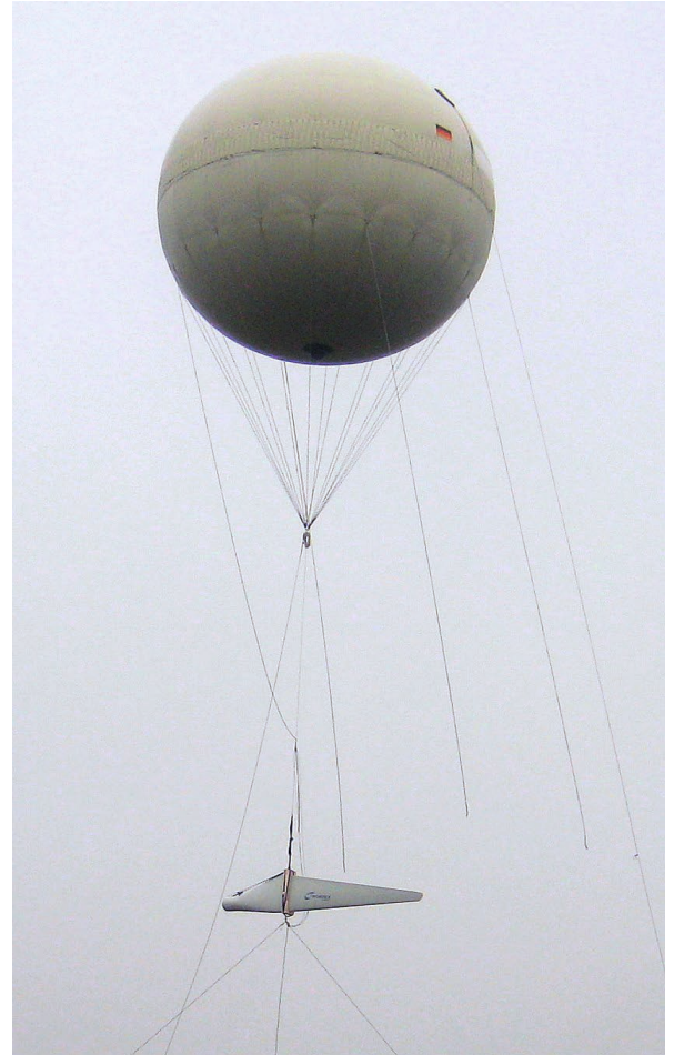
View ahead: CargoLifter crane balloon
