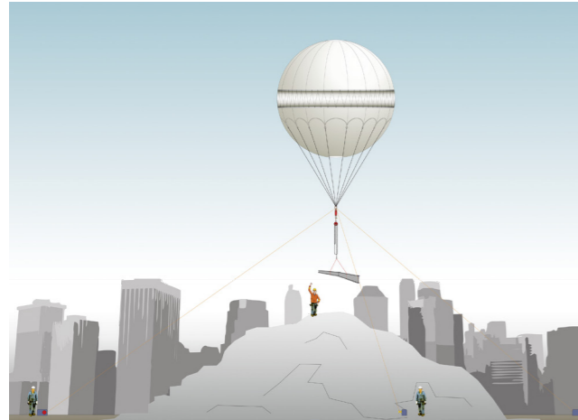
AirCrane working on instable ground
